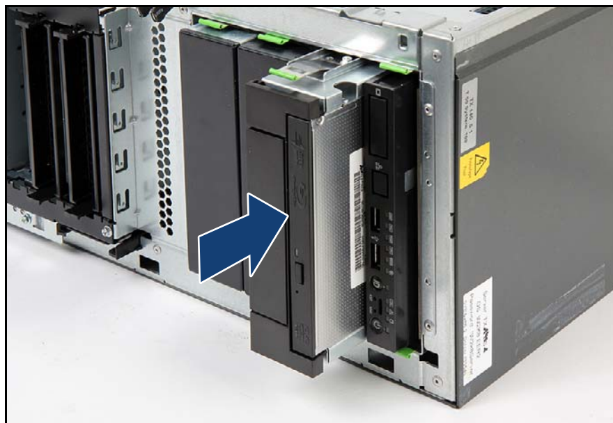
図 198: Installing the slimline drive
