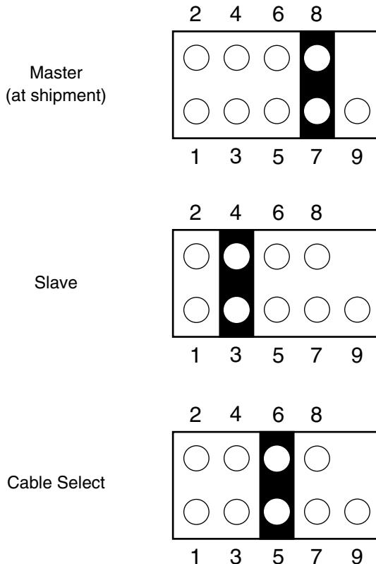
In Cable Select mode, the drive can be configured either master drive or slave drive.
