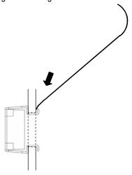
2. Push down the tool towards the cage nut and remove it.
