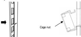
2. Insert the edge of tool from this side of a installation hole and hook the other edge of the cage nut.
