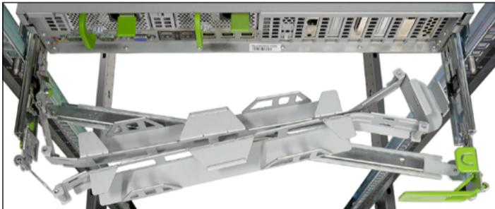
After installation, the CMA should lay on the crossbar, as shown in the picture.
