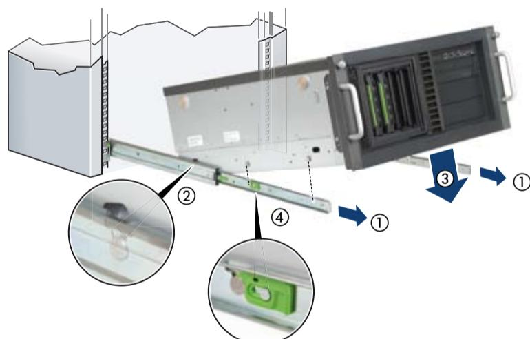
**!** Ensure that the safety lock has been inserted before the server is inserted (see the figure above)!
