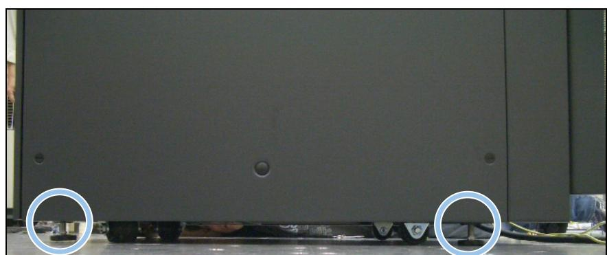
Install the adapters A3C40126894 on both sides of the system unit:
