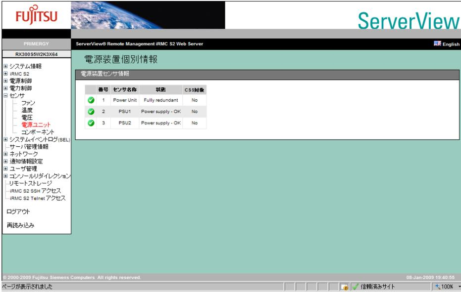
The screenshot shows the ServerView Remote Management interface for an IBM RX300S5W2K3X64 server. The main content area is titled '電源装置個別情報' (Power Supply Unit Individual Information) and contains a table of power supply unit sensor information.
