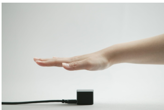
Palm vein sensor PalmSecure™ (35mmW×35mmD×27mmH)
