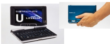
FMV-BIBLO LOOX U50XN (Sep/2007, The world's smallest convertible type PC, 555g in the lightest composition)
