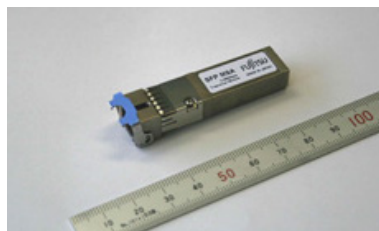
Compact optical transceiver for G-PON optical access
