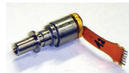
Laser module (TOSA) and 10-Gbps modulation
