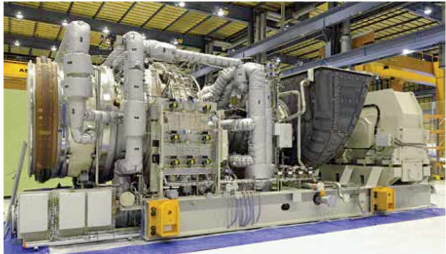
The picture shows the Siemens gas turbine SGT-800
