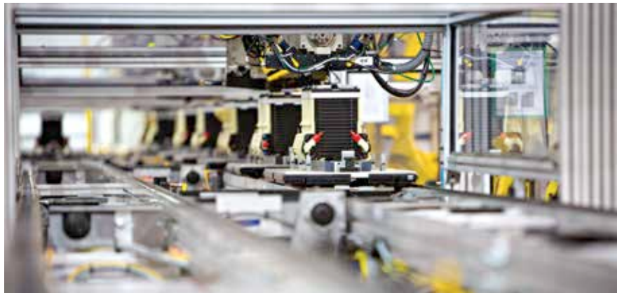
Ultrasonic welding, a high-tech process typically used in the aerospace and medical industries, helps ensure high quality for the new Cadillac ELR extended-range electric luxury coupe going on sale in North America in early 2014. General Motors' Brownstown Battery Assembly plant near Detroit uses ultrasonic welding to join metal electrode tabs on ELR's lithium-ion battery with precision accuracy and quality. The Brownstown battery plant uses an automated system to execute millions of these welds each year. (Photo by Jeffrey Sauger for General Motors)
