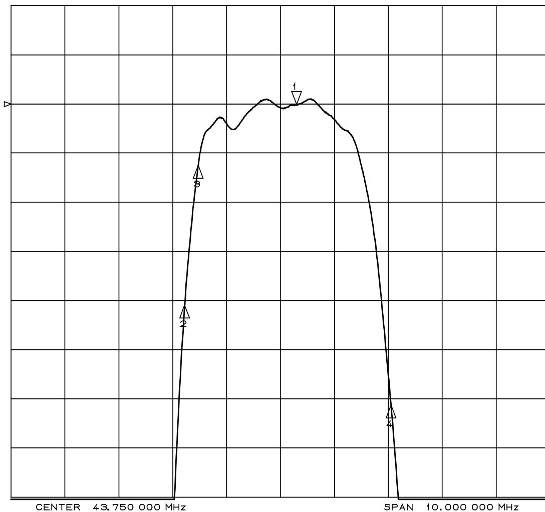
Amplitude Response (1dB/div)
